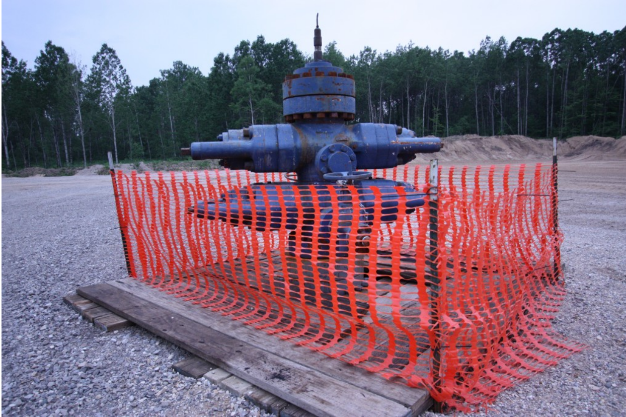
The Christmas tree at State Mancelona 1-28 HD1, a frack well in the state forest in Antrim County. Photo by LuAnne Kozma. Copyright by Ban Michigan Fracking.
